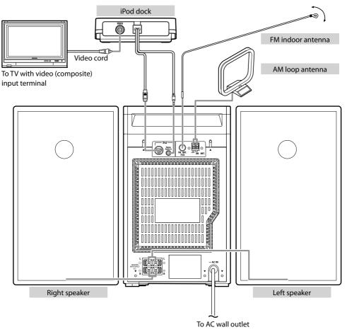
· Insert the plug firmly all the way into the AC wall outlet.
